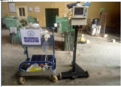
Figure 9: Completed mechanical ventilator unit with a monitor and solar panels
